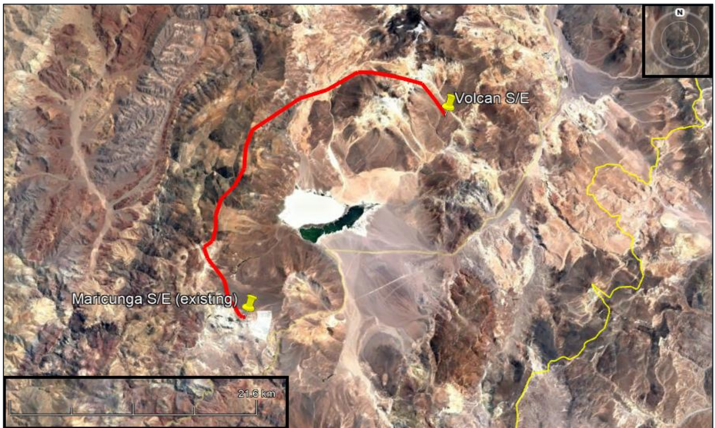
Figure 18-11: Proposed Transmission Line 110 kV Route.
