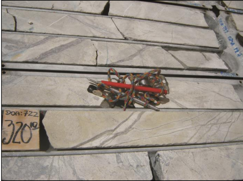
Figure 14-1: Example of Maricunga-style Veining and Stockworks, Volcan Project (Interval from 318.0-320.0 m grades 1.08 g/t Au, 0.10% Cu)
