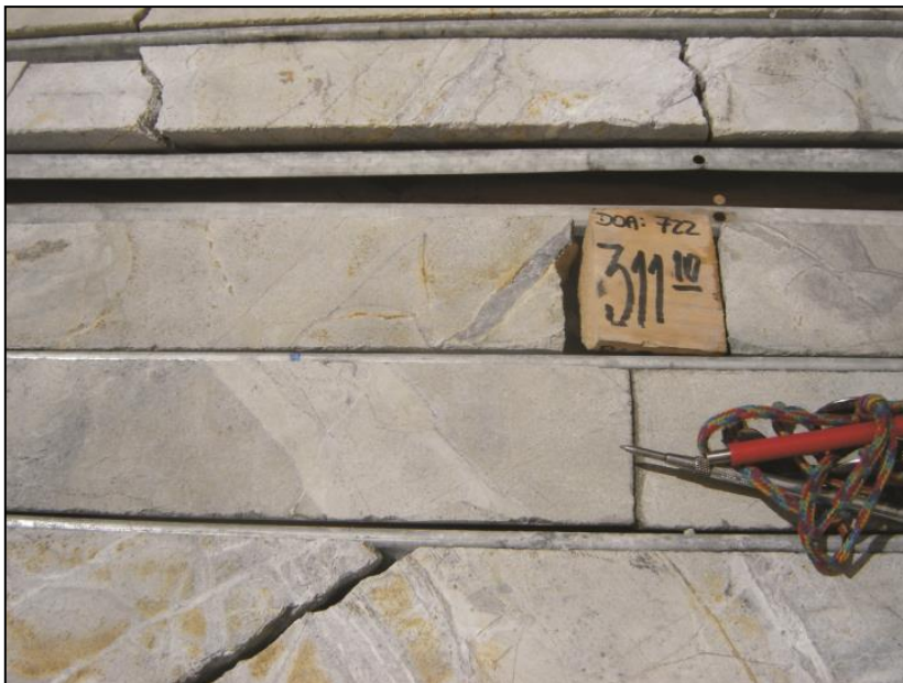
Figure 14-2: Example of Disseminated and Stringer Sulphide Mineralization, Volcan Project (Interval from 310.0-312.0 m grades 1.32 g/t Au, 0.15% Cu)
